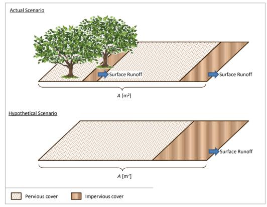
Figure 1 i-Tree Eco version 5 precipitation interception model diagram
