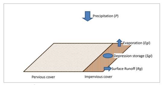
Figure 7 1<sup>st</sup> stage of the precipitation interception by impervious cover, starting when the precipitation (*P*) starts and ending when the depression storage of impervious cover (*Sgi*) reaches  $Si_{max}$
