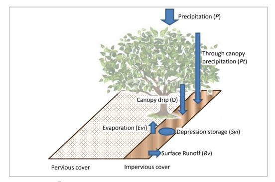
Figure 5  $1^{st}$  stage of the precipitation interception by impervious cover, starting when the precipitation (*P*) starts and ending when the depression storage of impervious cover (*Svi*) reaches *Si<sub>max</sub>*
